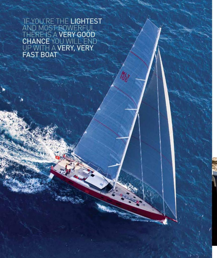
Nomad IV's deck plan follows the principles applied to the design of IMOCA 60s and other shorthanded racing yachts, so a crew of just four can safely handle her sailplan. Her wide aft beam means a giant cockpit for guests to enjoy, with tables either side that convert to sunpads (below)
