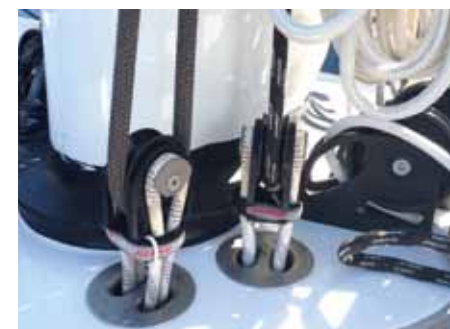
▶ Right: open blocks at the mast step allow halyards to be led to either of two winches. ▶ Far right: the engine and machinery room. In the foreground, the grey pipes are the carbon water ballast pipes with valve shut offs, pneumatic system to the left, watermaker, genset and engine behind
