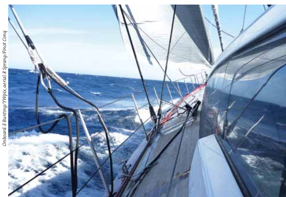
▼ Below: spray flies off the leeward bow as we reach out beyond the Porquerolles under reefed mainsail and J2. As you can see here, the FC100 has carbon standing rigging, though Kevlar backstays
